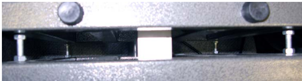
Figure 3-1. Overload Stops on Defender E Base
